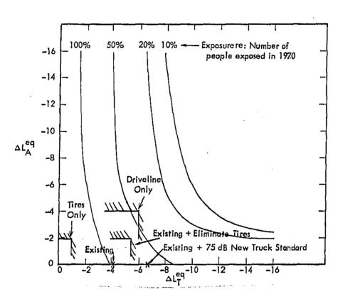
Figure 15. Limitation of Low-Speed Exposure Reduction in 2000 if One Source Component Is Reduced.
