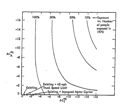
Figure 14. Vehicle Noise Reductions Required to Reduce High-Speed Exposure in 2000.
