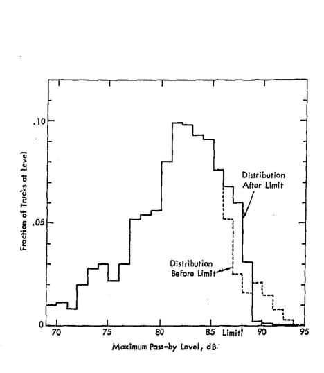
Figure 3. Effect of Operating Limit on Truck Noise Level Distribution
